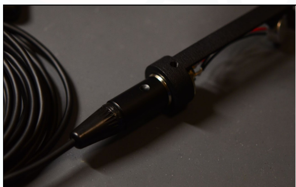
2.6 & 2.7 - Soldering the mic capsule leads and attaching the Mini XLR panel mount...
