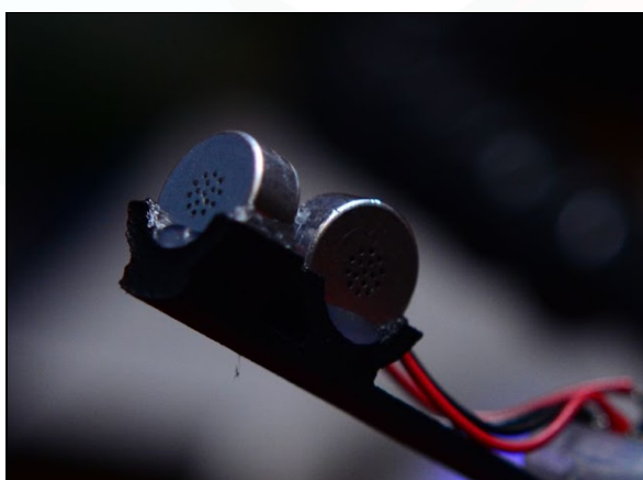
2.8 - Gluing the capsules in place...
